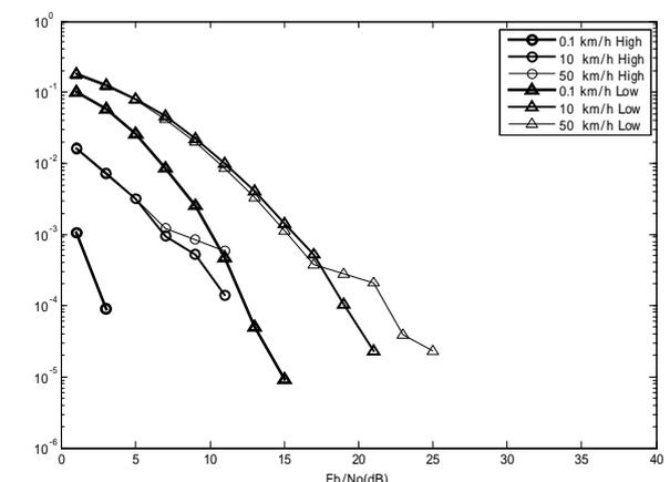
Fig. 8 TRAP Probability of Bit Error (K=5)
