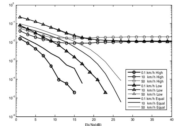
Fig. 7 TRAP Probability of Bit Error (K=0)
