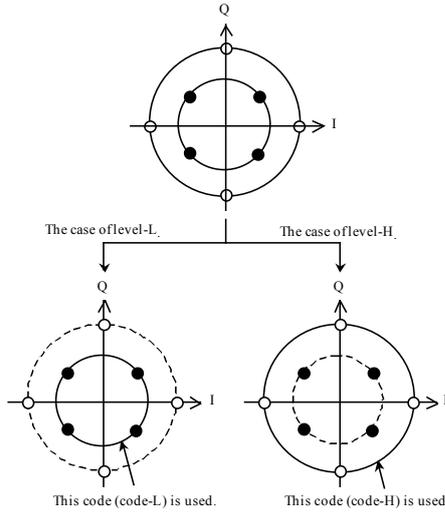
Fig. 3. The proposed concept to realize UEP for 2 levels of importance.
