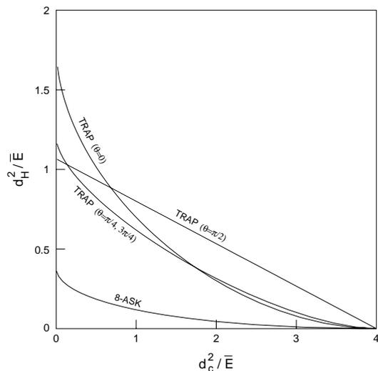
Fig. 3: The signal spacing of the H code ( $d_H^2$ ) versus the minimum code spacing ( $d_c^2$ ) for  $\beta = 1/\sqrt{2}$ .
