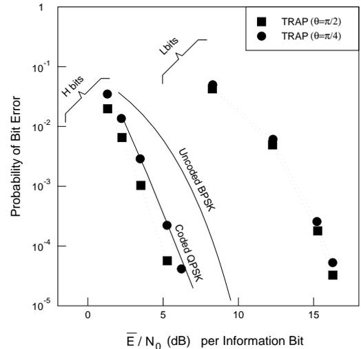
Fig. 6: The performance of the proposed UEP scheme.  $d_c^2/\bar{E} = 0.3$  and  $\beta = 1/\sqrt{2}$ .
