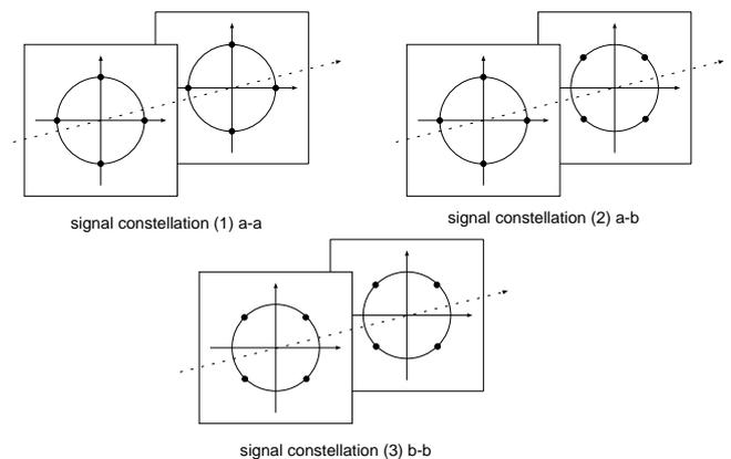
Fig. 3: An example of four–dimensional signal constellations for use with three importance levels
