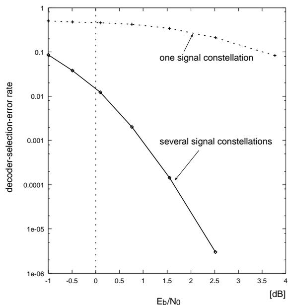
Fig. 4: Decoder-selection-error rate
