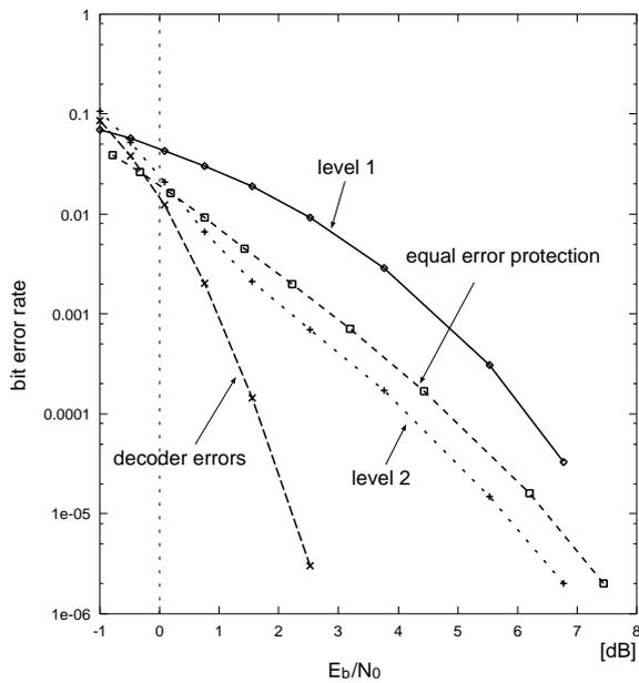
Fig. 5: The bit error rate performance of the proposed system
