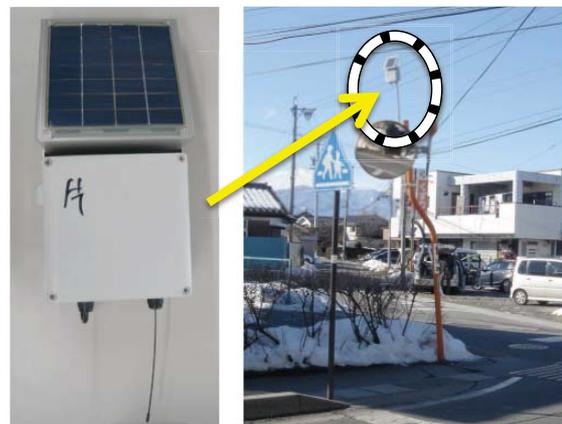
Figure 2: Ad-Hoc network transponder (left) and installation appearance (right)
