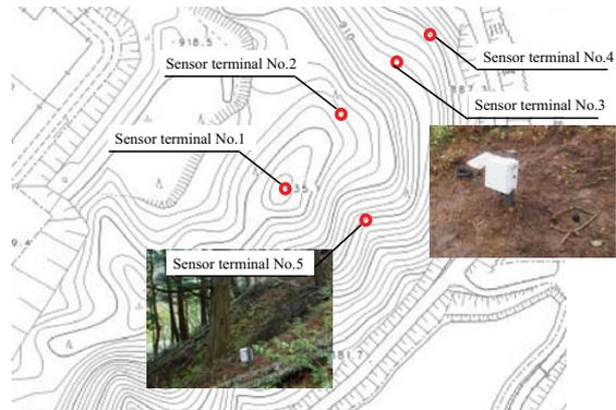
**Figure 4: Landslide sensor terminal installed in the mountains of Shiojiri City (in 2012)**
