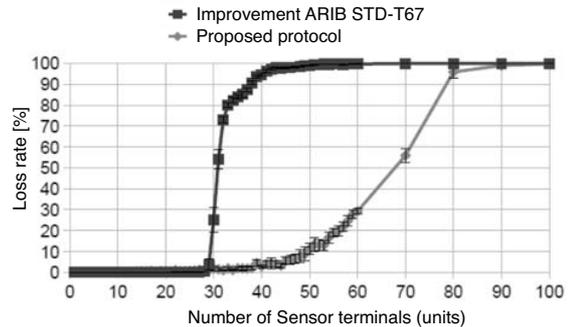
**Figure 5: Comparison of loss rates for conventional protocol and proposed protocol**
