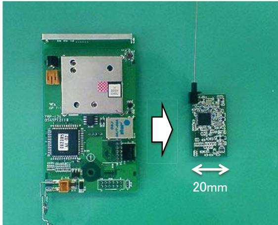
**Figure 3: Wireless circuit currently in use (left), and prototype wireless module (right)**
