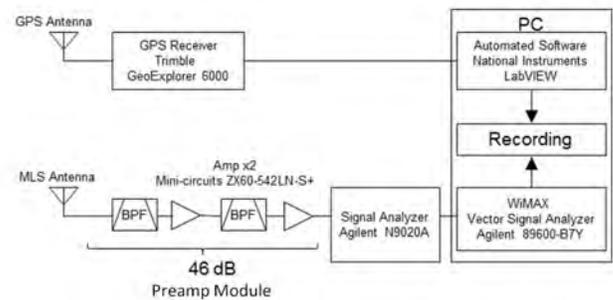
Fig. 5. Block Diagram of Rx System
