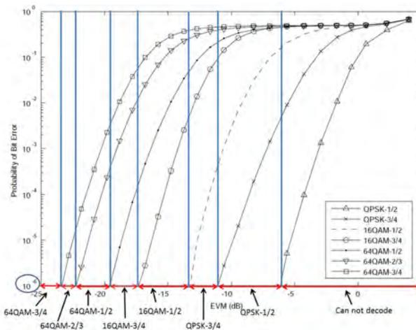
Fig. 1. EVM v.s Bit Error Rate by computer simulation
