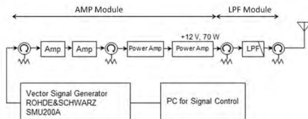
Fig. 3. Block Diagram of Tx System
