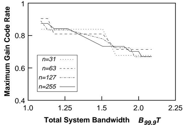
Fig. 4. The code rate at which the maximum gain is achieved for BCH codes as a function of the total system bandwidth for various block lengths  $n$ .
