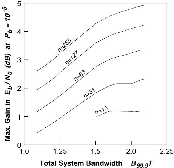
Fig. 5. The maximum gain, relative to the uncoded system, in SNR achieved at a bit error rate of  $10^{-5}$  using ideal block codes as a function of the total system bandwidth for various block lengths  $n$ .
