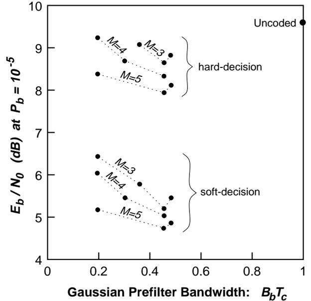
Fig. 6. The SNR required to achieve a bit error rate of  $10^{-5}$  as a function of the normalized Gaussian prefilter bandwidth,  $B_bT_c$ , for various convolutional codes with  $M$  memory elements decoded using hard and soft decision Viterbi decoding. The total system bandwidth is equal to  $B_{99.9}T = 2.05$ , which corresponds to an uncoded system with  $B_bT = 1.0$ .
