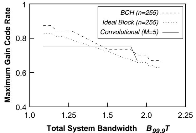
Fig. 8. The code rate at which the maximum gain is achieved as a function of the total system bandwidth for different types of codes.
