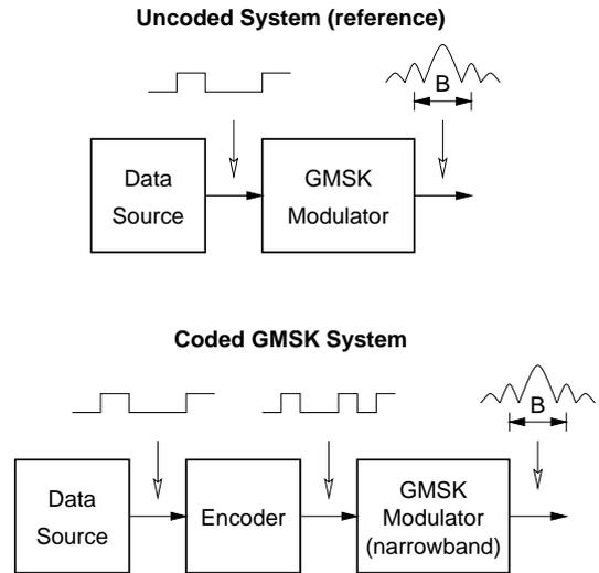
Fig. 1. The coded GMSK system examined in this paper compared to the uncoded system used as a reference.
