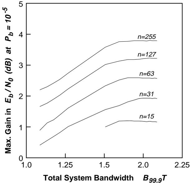
Fig. 3. The maximum gain, relative to the uncoded system, in SNR achieved at a bit error rate of  $10^{-5}$  using BCH codes as a function of the total system bandwidth for various block lengths  $n$ .
