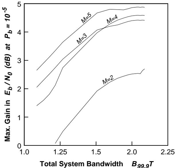
Fig. 7. The maximum gain in SNR achieved at a bit error rate of  $10^{-5}$  for soft-decision decoded convolutional codes as a function of the total system bandwidth for various numbers of memory elements  $M$ .
