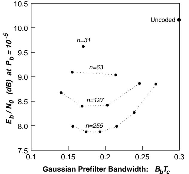
Fig. 2. The SNR required to achieve a bit error rate of  $10^{-5}$  as a function of the normalized Gaussian prefilter bandwidth,  $B_b T_c$ , for various BCH codes with block length  $n$ . The total system bandwidth is equal to  $B_{99.9} T = 1.167$ , which corresponds to an uncoded system with  $B_b T = 0.3$ .
