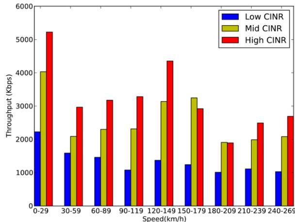
Fig.3. Moving Speed and Throughput.
