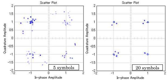
Fig.10. Scatter plot with the initial tap gains.
