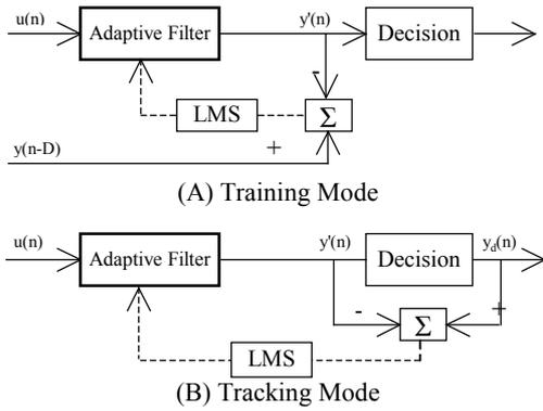
Fig.5 The structure using a LE [2].
