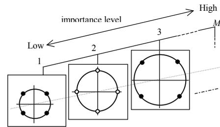
Fig.3 Multilevel trellis coding to realize UEP.
