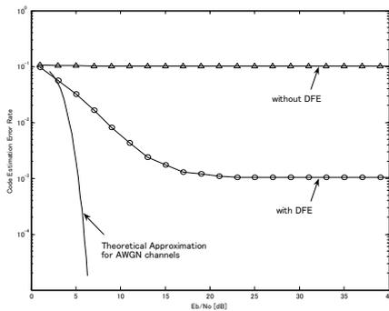
Fig.9. Code estimation error rate versus  $E_b/N_0$ .
