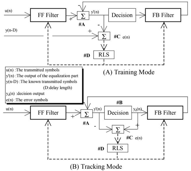
Fig.6 The structure using a DFE.
