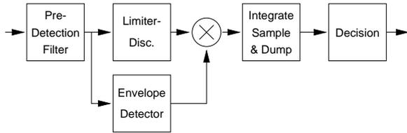
Fig. 3. The FM-ISD processor.
