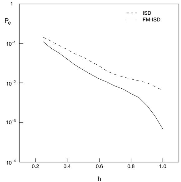
Fig. 5. Performance comparison of the ISD and FM-ISD processors as a function of  $h$  for the rectangular pulse shape,  $\overline{SNR} = 47dB$  and  $B_f T = 0.2$ .
