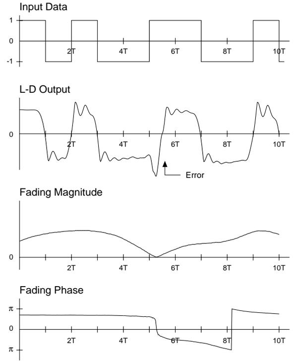
Fig. 2. Distortion of baseband signal due to fading and ISI.
