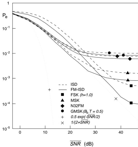
Fig. 6. Performance of the FM-ISD Processor for  $B_f T = 0.05$ .
