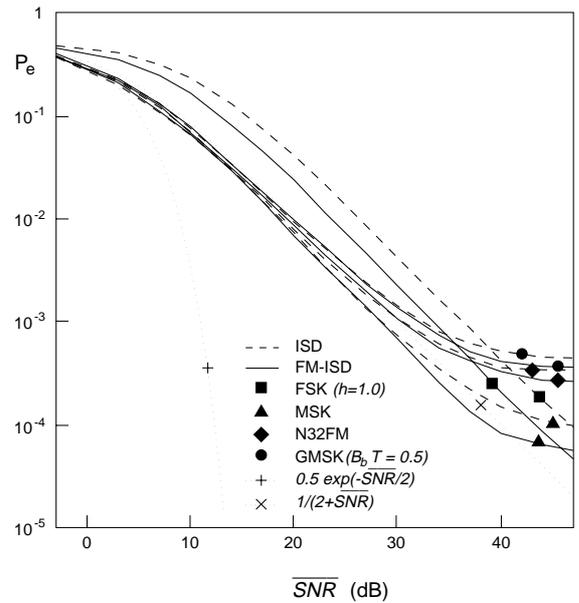
Fig. 7. Performance of the FM-ISD Processor for  $B_f T = 0.01$ .
