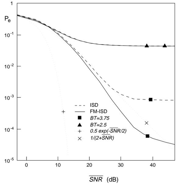
Fig. 9. Performance of the ISD and FM-ISD processors using a 20th order Butterworth pre-detection filter for FSK ( $h = 1.0$ ).
