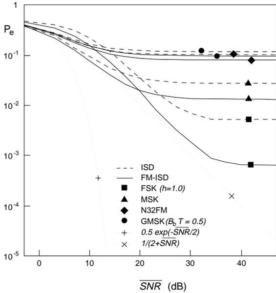
Fig. 4. Performance of the FM-ISD Processor for  $B_f T = 0.2$ .
