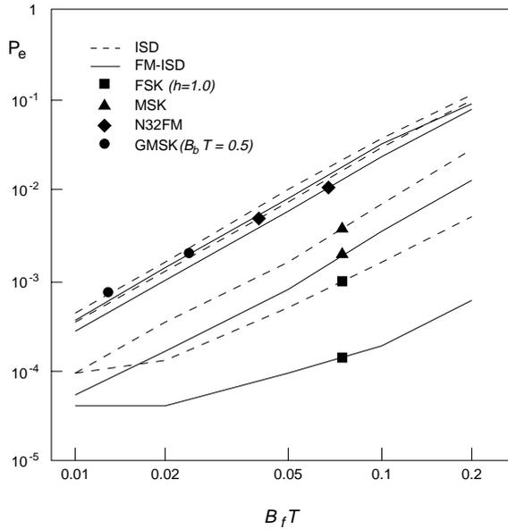
Fig. 8. Performance comparison of the ISD and FM-ISD processors as a function of fading rate for  $\overline{SNR} = 47dB$ .
