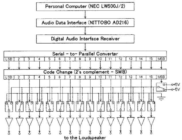
FIG. 11. Block diagram of the PCM driving circuit.
