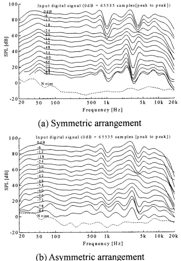
FIG. 15. Frequency responses of the digital loudspeaker at a distance of 10 cm from the center of the diaphragm. The dashed lines show the ambient noise level.
