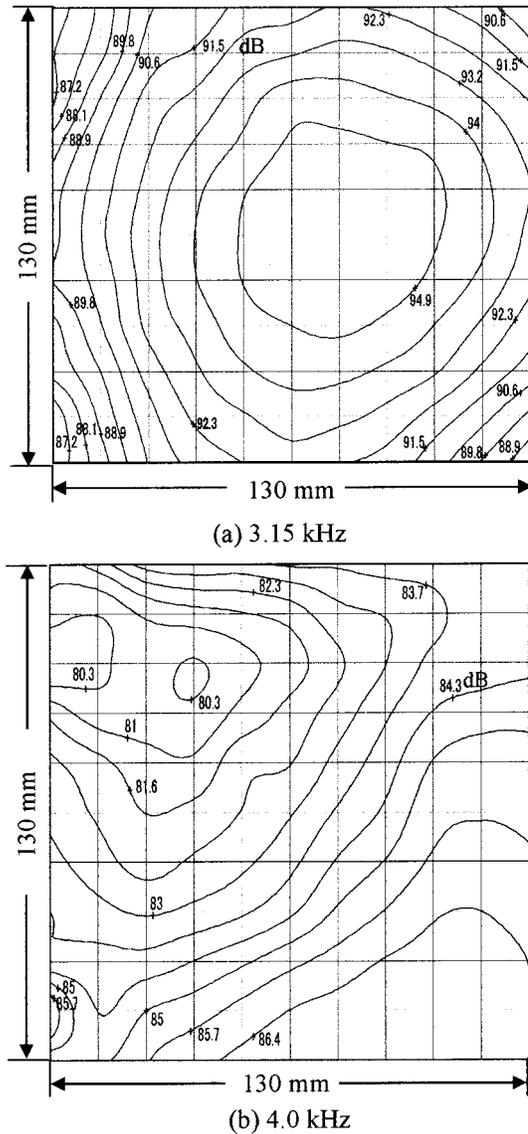
FIG. 17. Distribution of the sound intensity level (dB *re*:  $10^{-12}$  W/m<sup>2</sup>) at a distance of 10 cm from the front of the diaphragm.
