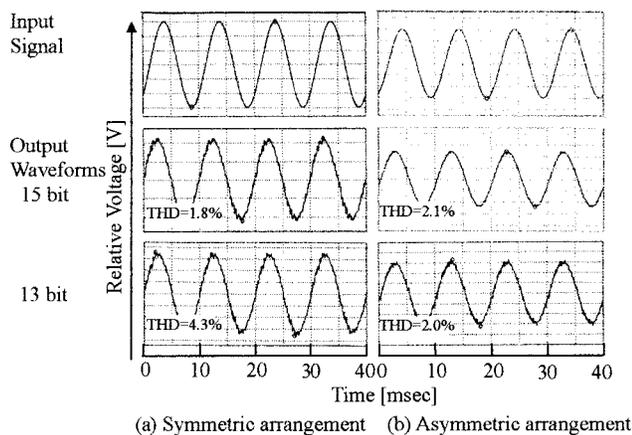
FIG. 13. Output waveforms from the electrodynamic planar digital loudspeaker at 100 Hz.
