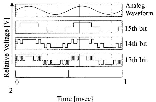
FIG. 12. Output waveforms of our PCM driving circuit.
