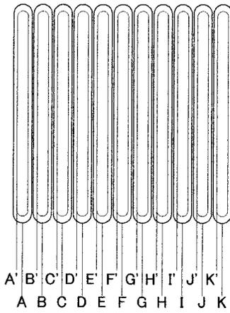
FIG. 3. The 22 voice coils in our electrodynamic loudspeaker.
