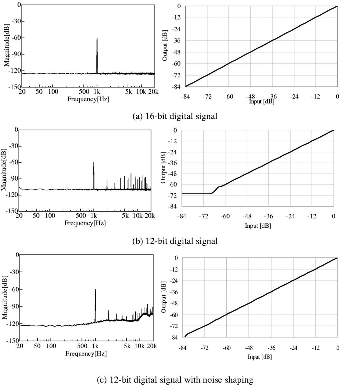
FIG. 3. The frequency response and linearity characteristics of the noise shaper when the following digital signals are input: (a) 16 bit digital signal, (b) 12 bit digital signal, and (c) 12 bit digital signal with noise shaping. The figures on the left are the frequency responses to a 1 kHz pure tone (-60 dB), while the figures on the right are the linearity characteristics at 1 kHz.
