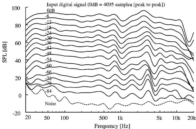
FIG. 8. Frequency response of the digital loudspeaker driven by a 12 bit digital signal with noise shaping at a distance of 10 cm from the center of the diaphragm. The dashed lines show the ambient noise level.
