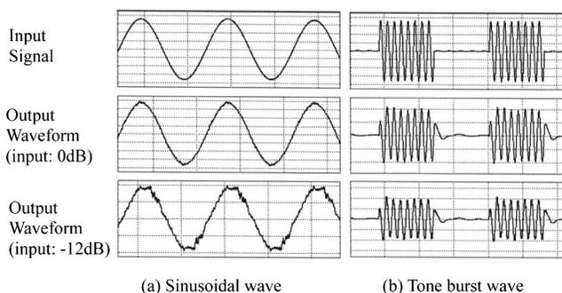
FIG. 7. Output wave forms from our electrodynamic planar digital loudspeaker driven by (a) a pure tone signal (12 bit: 0 dB, and 10 bit:  $-12$  dB) and (b) a tone burst signal (12 bit: 0 dB, and 10 bit:  $-12$  dB) at 100 Hz.
