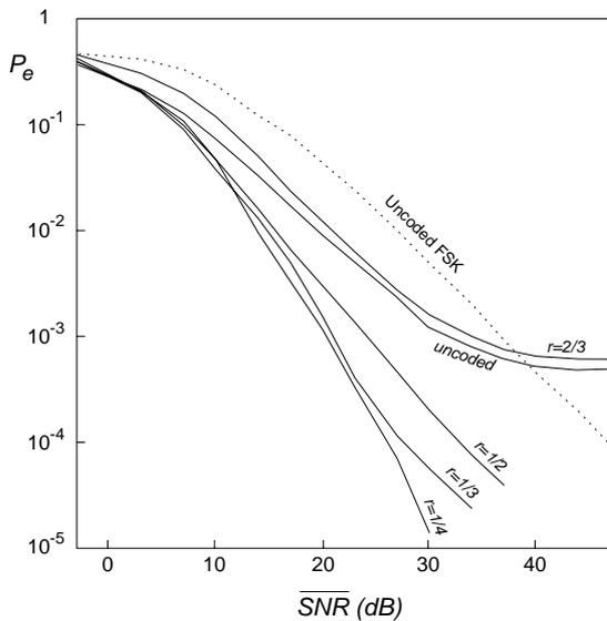
**Fig. 3** Performance of coded GMSK for  $B_f T = 0.01$  using 4-state codes.  $r$  is the code rate.
