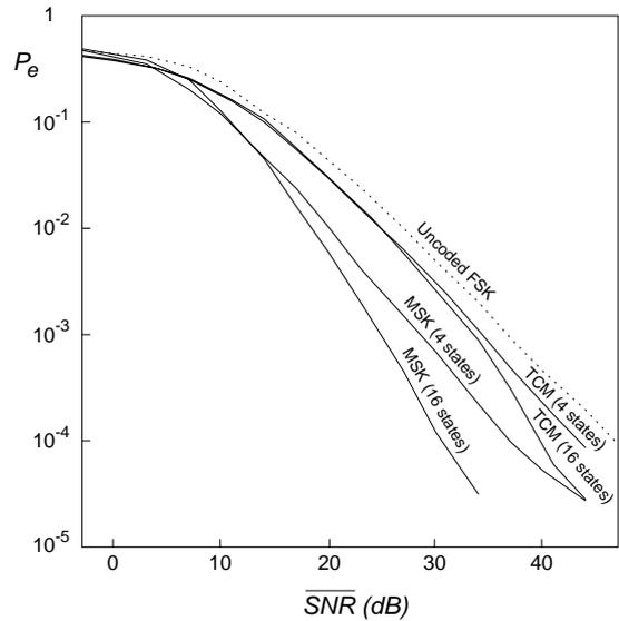
**Fig. 4** Performance comparison of MSK ( $r = 2/3$ ) and TCM using 4 and 16 state encoders for  $B_f T = 0.01$ .
