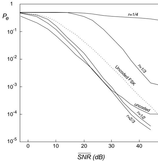
**Fig. 2** Performance of coded MSK for  $B_f T = 0.01$  using 4-state codes.  $r$  is the code rate.
