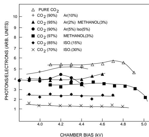
Fig. 2. Ratio of photons and anode pulse amplitudes.
