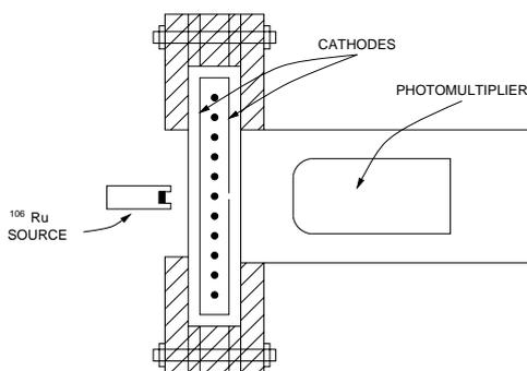
Fig. 1. The wire chamber and photomultiplier.
