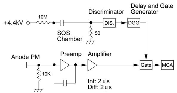
Fig. 4. Photon pulses gating and measurement.
