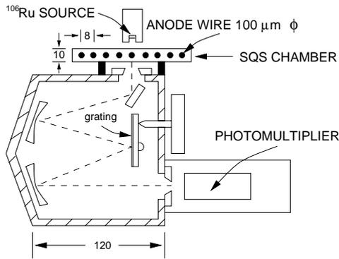
Fig. 3. Monochromator and wire chamber assembly.
