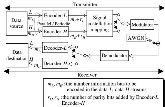
Fig. 3. Coded modulation with time multiplexing [8,9]
