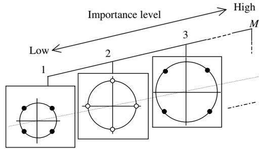
Fig. 5. Multilevel Trellis coding to realize UEP for  $M$  levels of importance
