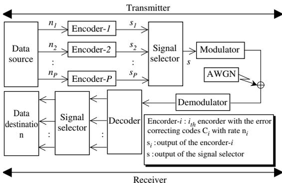
Fig. 1. Multilevel encoder [7]
