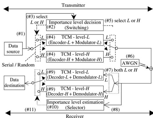
Fig. 4. The proposed UEP scheme in AWGN channels for two levels of importance
