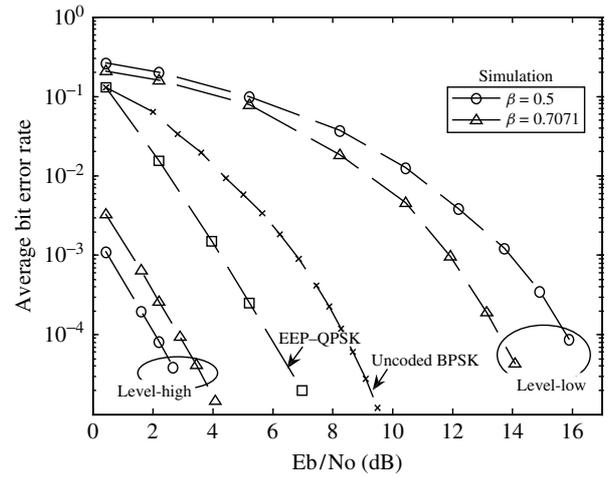
Fig. 13. Average bit error rate versus  $E_b/N_0$  ( $N = 30$ )
