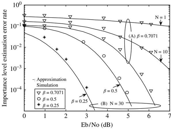
Fig. 12. Importance level estimation error rate versus  $E_b/N_0$
