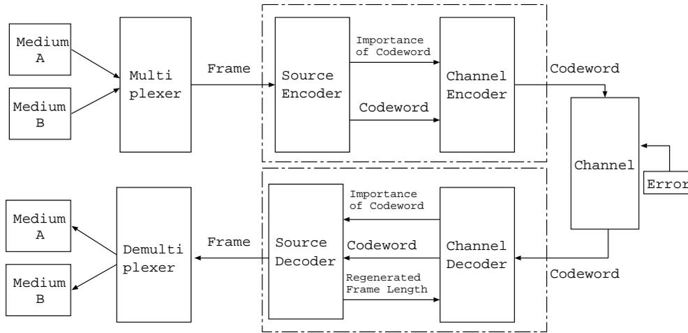
Figure 5: A combined source and channel coding system.
