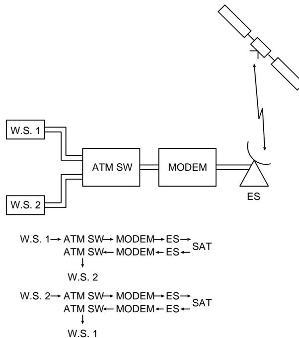
Figure 1: Intelligent Communication Experimental System
